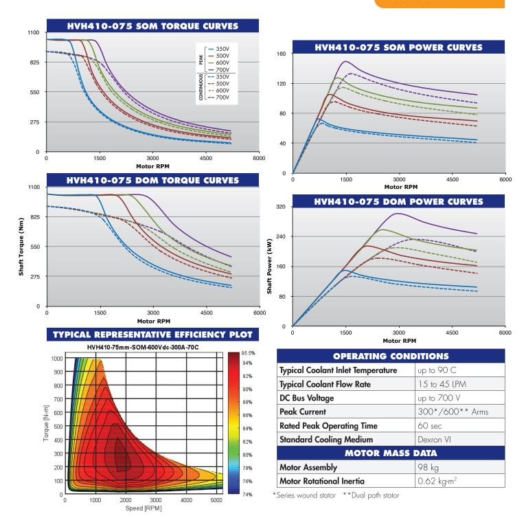
Note: Graphs above are based on actual test data. The torque and power ratings are based on typical operating conditions as noted on the performance graphs. There are several variables that may change the motor performance, including coolant flow rate, operating temperature, inverter settings and parameters, etc. For actual performance, the motor must be evaluated in its final system and application. All specifications are subject to change.
