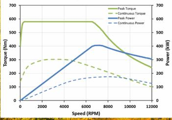
Being the higher-powered version of the iM-225, the iM-375 is built using the CM350 inverter and HVH250 motor core. This integrated module packs a 580Nm punch within a compact package and has a peak power of 400kW (537hp) at 700Vdc. It's loaded with integrated features like an oil pump, oil cooler, oil sump and water pump.
